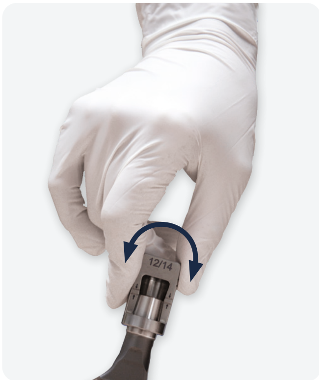
Figure 6 Testing the clamp connection
