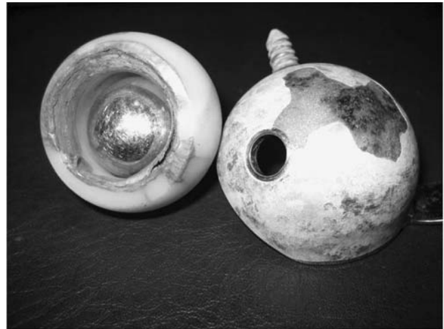
Fig. 3 Aspect of the acetabular cup system after intraprostatic dislocation. In this case the intraprostatic dislocation is associated with loosening of the acetabular component
